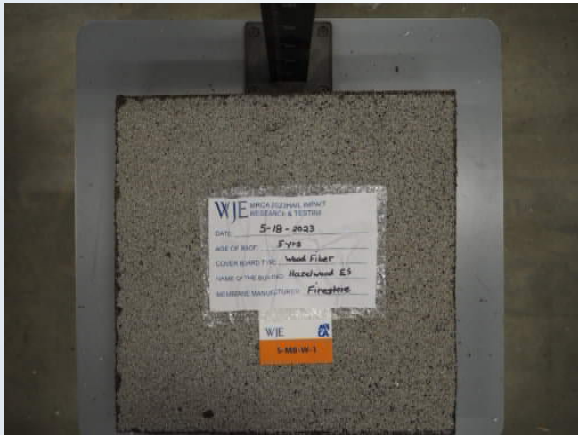
5 and 10 year old samples wood fiber cover board (Jim Ramser, T&R member )
