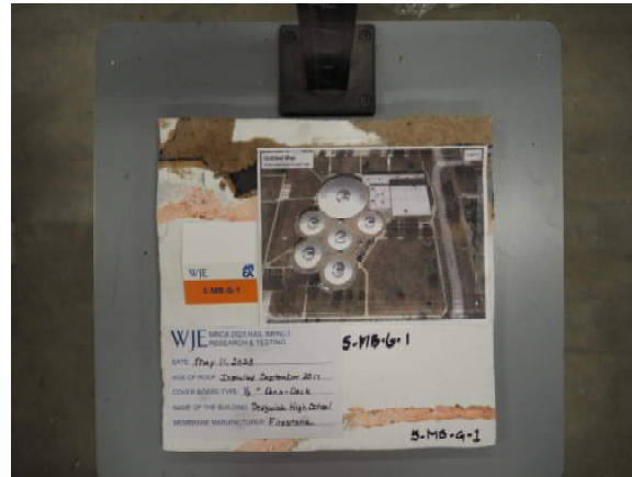
5 and 10 year old samples gypsum cover board (Kurt Steinkuhler, T&R member )
