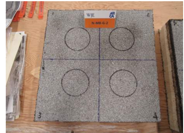
New samples gypsum/wood fiber cover board (Chris Daly, T&R member )
