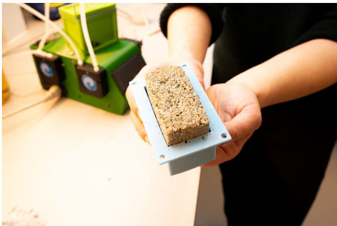
The mixture of bacteria and sand in the mould is fed with finely ground limestone that is partially dissolved by another bacteria and a solution containing urea. Interaction of the two bacteria causes calcium carbonate crystals to precipitate, and these bind the sand grains together. After drying, a small brick of concrete is removed from the mould. Photo: Håvard Egge.
